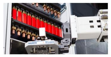
Virtually unlimited number of magazine locations The technology of the Robot Dynamic 150L allows up to 10,000 magazine locations for pallets, electrodes and palletized fixtures. The limit is only the available space conditions.
