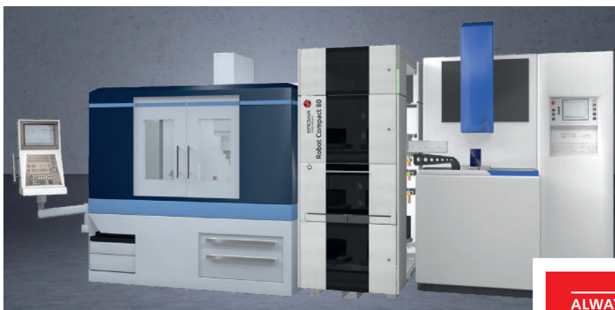
EROWA Robot Compact 80 between an EDM machine and a milling center.
