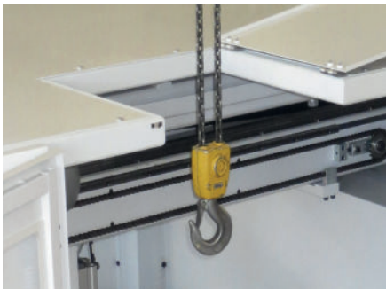
Top loading door for crane operation.
